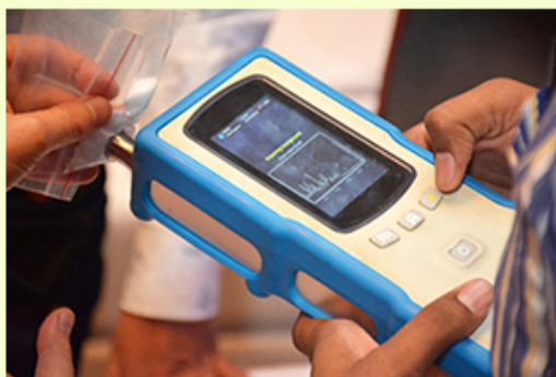
A typical "paperback book" form factor handheld instrument, NanoRam portable Raman from B&W Tek. (Picture courtesy of B&W Tek)
