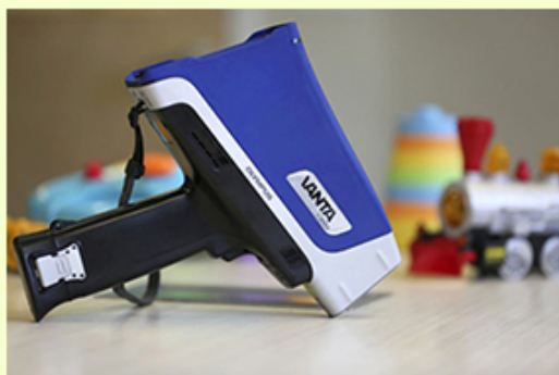
A typical "cordless drill" form factor handheld instrument, Vanta portable XRF from Olympus. (Picture courtesy of Olympus)
