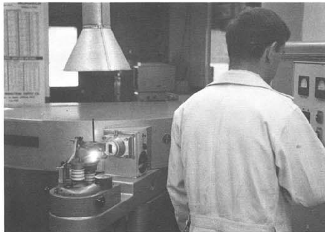
It's not 218 Alloy if magnesium volatilizes from the die cast pot! This and other problems such as mixed stock, out of spec, iron content too high are some of the production perils that arise if close control is not maintained on incoming and in-process materials. Mike Buyaki checks out the Spectrophotograph preparatory to auditing a vendor certification.
