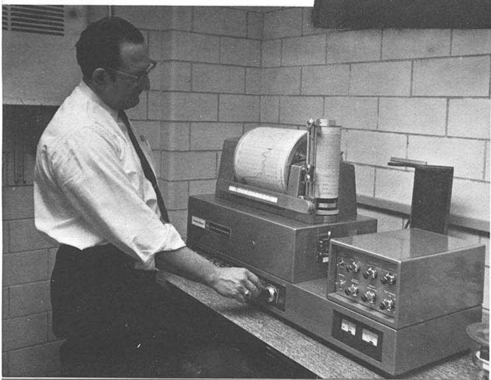
The infrared spectrum of a polymeric coating is obtained by R. J. Hansen using the Perkin-Elmer Model 421 Dual Grating Spectrophotometer.
