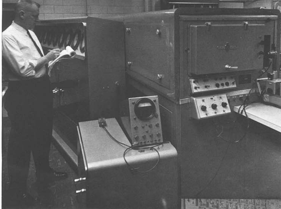
Quantitative analysis of a can making alloy is conducted by H. M. Wilson on the Baird Atomic 3-Meter Research Direct Reading Spectrograph.
