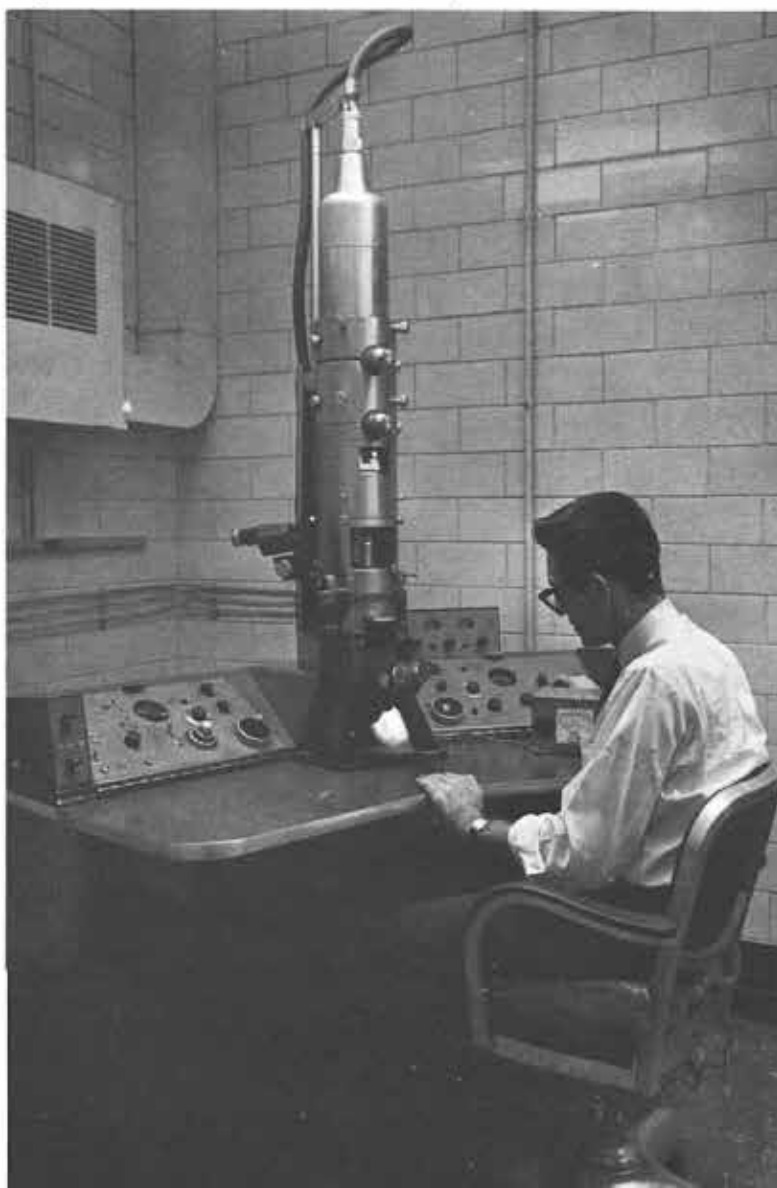
J. J. Brynes examines a vacuum metallized surface using the RCA EMU-3 Electron Microscope.
