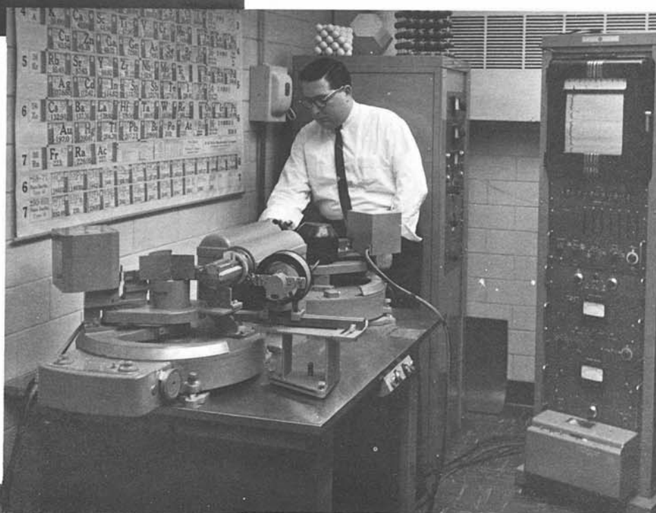
J. A. Sheinkop uses the GE X RD-5 X-Ray Spectrograph for elemental analysis of a glass.
