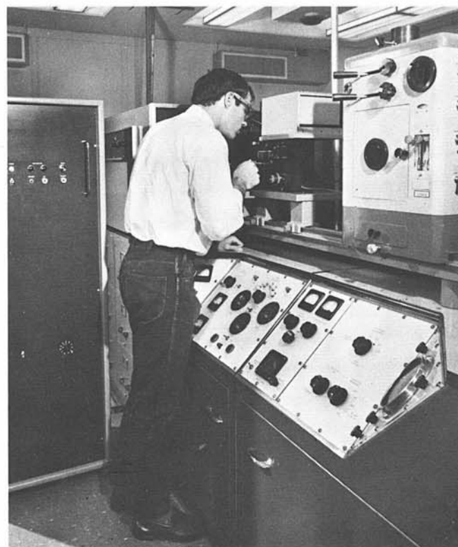
Mr. Daniel Marcellus, a college student and a participant in the Bureau's summer research program, uses a laser probe as the light source in the process of analyzing a micro-sample. The laser is mounted on a 3.4-meter Ebert Spectrograph. The Section also has two other large spectrographs.
