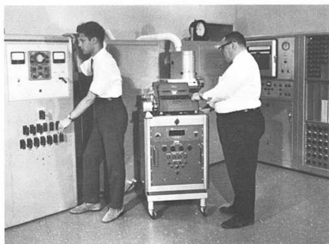
Mr. Gerald Wolfson (left) studies the discharge pattern of this large emission spectrometer. Mr. Doward Bouchette checks results as they are printed at the readout. This complex of equipment at NBS pioneered in completely computerized emission spectrometry.
