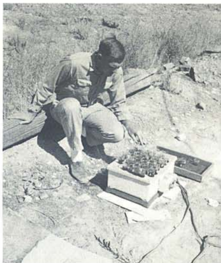
Gordon Van Sickie, chemist on the team, is putting rock samples in a final solution prior to atomic absorption analysis to determine gold content.
