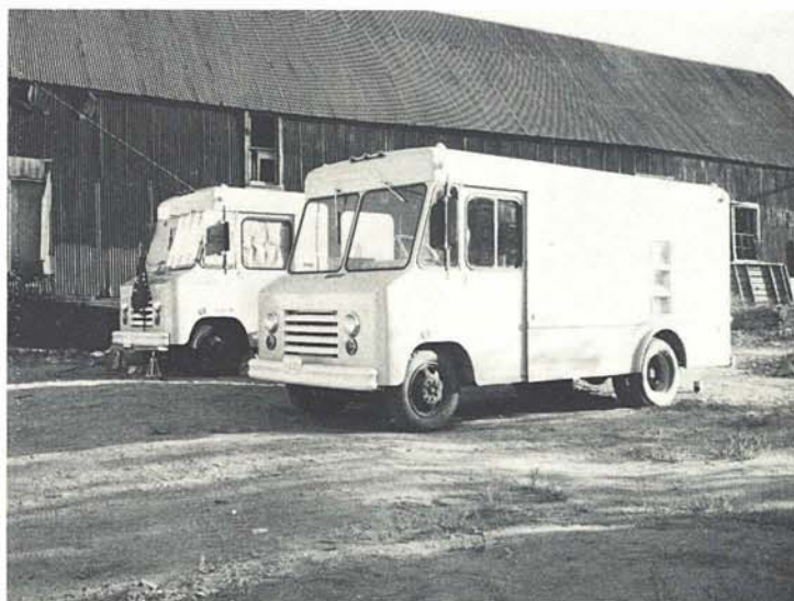
For field trips into areas that are relatively easy to enter these two laboratory vans are used together. Two men, one per truck, make the trip with these units. The weighing room, darkroom and office are housed in one (foreground), and the spectrographic laboratory in the other.
