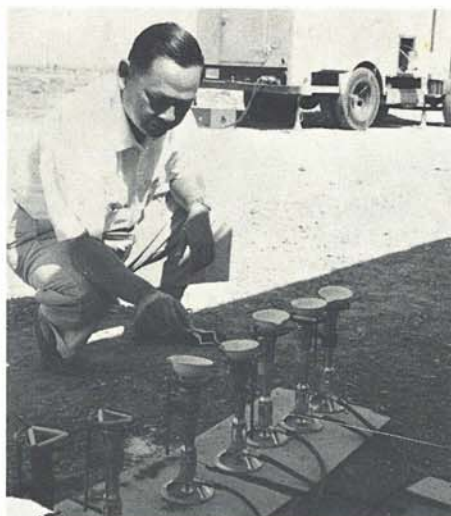
Kam Wo Leong, chemist, ignites samples of rock prior to gold analysis by atomic absorption.
