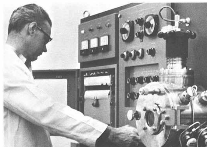
Technician W. Peterson measures transformation kinetics of steel samples on a high-speed dilatometer.
