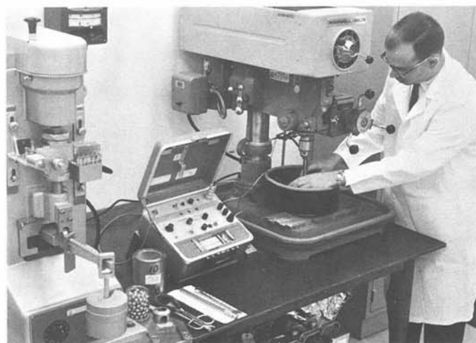
T. J. Risdon studies the effectiveness of molybdenum disulfide additive to cutting fluids. The instrument at the far left is a four-ball wear tester.
