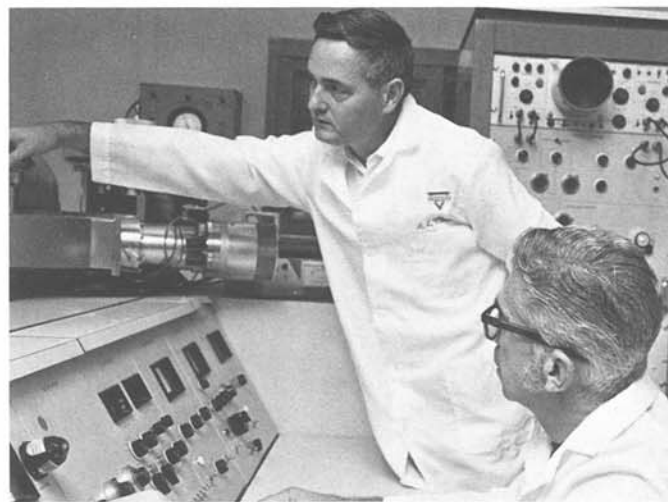
Mr. Dallas Winter (standing) and Mr. Knox Moore record high resolution mass spectra on photoplates as materials are eluted from GLC inlet.
