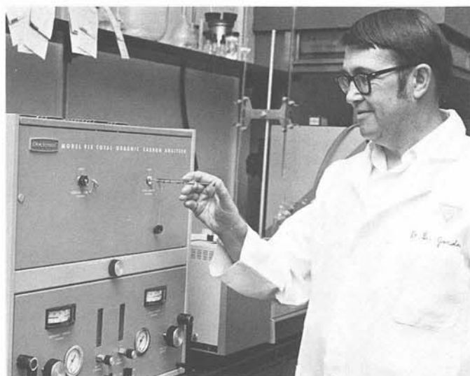
Dr. Donald E. Jordan injects a sample of water into the Beckman TOC (total organic carbon) analyzer.
