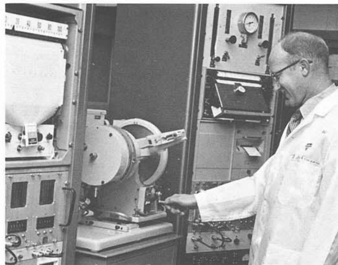
Mr. Charles F. Maddox measures the total and organic carbon content on the Leco Model TC-12 analyzer.
