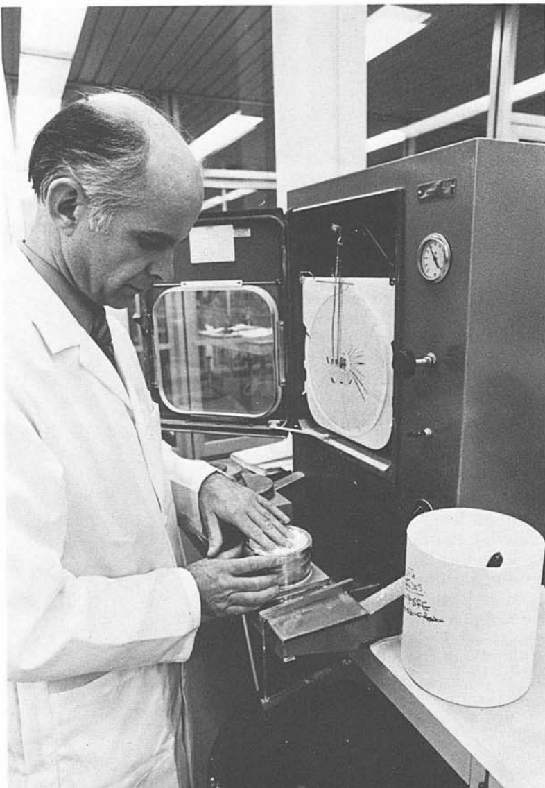
J. D. Zwicker prepares a powder specimen in the shear cell of the Jenike Flow Factor Tester for subsequent shearing to determine the relationship between consolidating pressure and strength. The values are used to assess flowability and to design bins.
