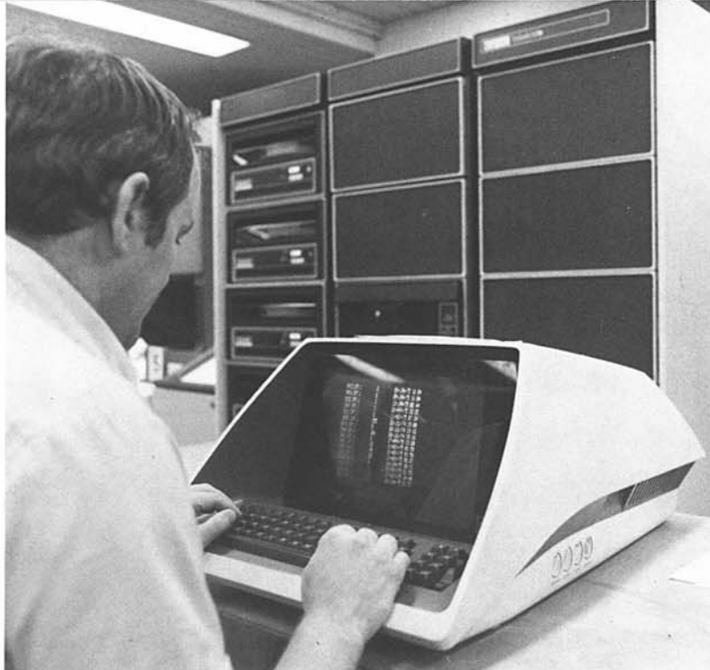
The results received at the midicomputer from the minicomputer are used for batch making, for the control of operations in the casting plant and for inventory purposes. D. Larouche is shown here working on a batch composition with the help of the DEC PDP11-40 midicomputer shown in the background.
