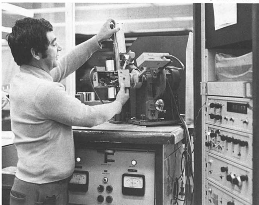
The control of the smelting process in the potrooms is done through the analysis of the electrolytic bath in each of the pots. The concentrations of some of the chemical constituents in the bath are measured with the help of an X-ray diffraction instrument controlled by a computer. Robert Pineault is shown here installing a tray of samples in the automatic sample feeder on the X-ray diffractometer.
