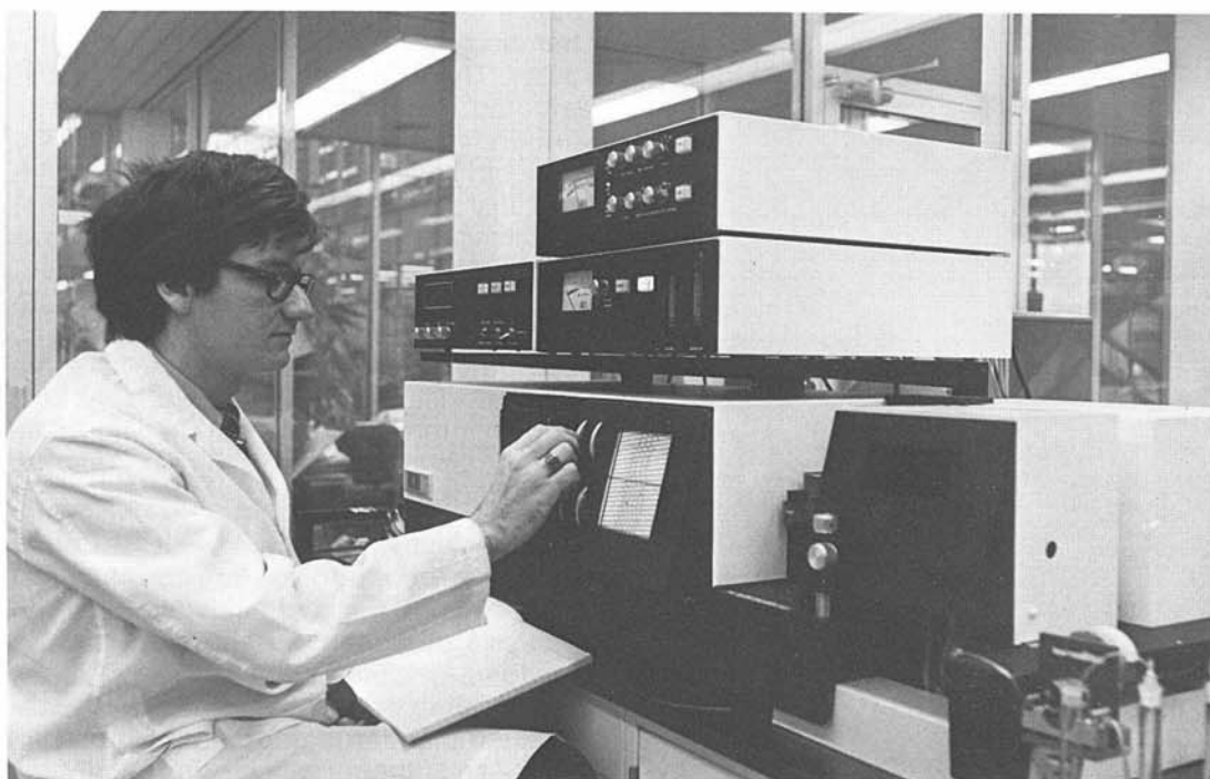
Mr. G. Dubé selects a suitable spectral line on the Spectraspan emission spectrograph, which uses a plasma source for exciting the elements from an atomized sample solution. Both qualitative examination and quantitative determination – down to low trace levels – can be quickly accomplished in many materials for all the elements normally determined by emission analysis.
