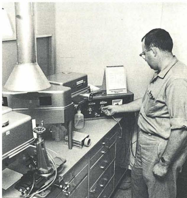
Richard A. Martin adjusts the Perkin-Elmer 214 atomic absorption spectrophotometer. Flip-chart on the console is to remind occasional operators of steps to follow.
